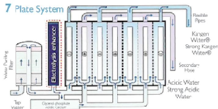
Figure 3: The scheme representation of electrochemical processes of water treatment in the Kangen ionizer
