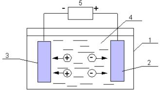
Figure 2: Scheme of the electrolysis cell: 1 – the case; 2 – anode; 3 – cathode; 4 – interelectrode space; 5 – DC power source.
